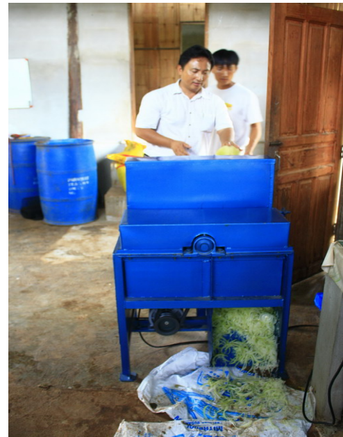
Abel demonstrating how to use the banana tree slicing machine to house parent
